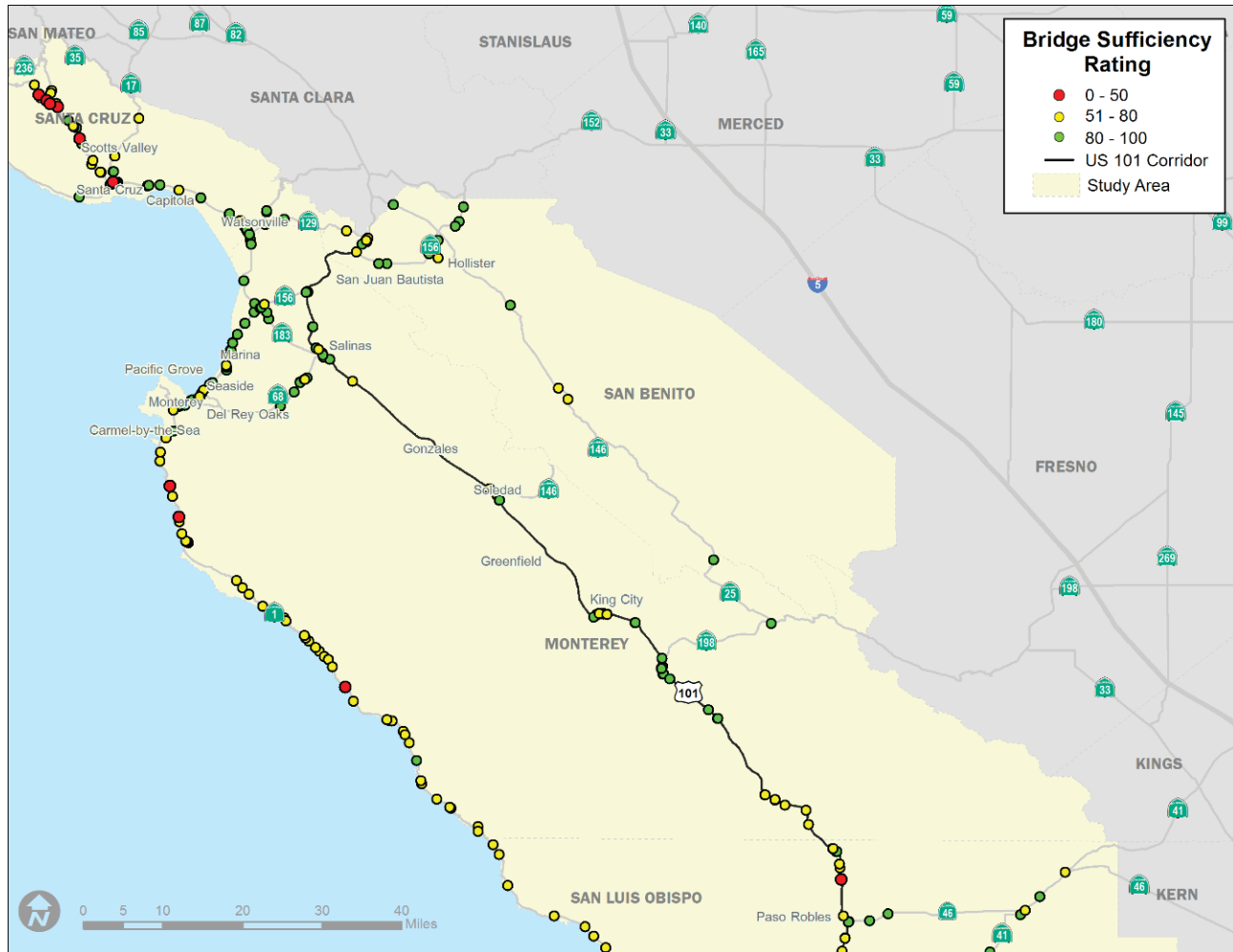
Figure 3.13 Bridge Conditions in Study Area Santa Cruz, San Benito, and Monterey Counties
