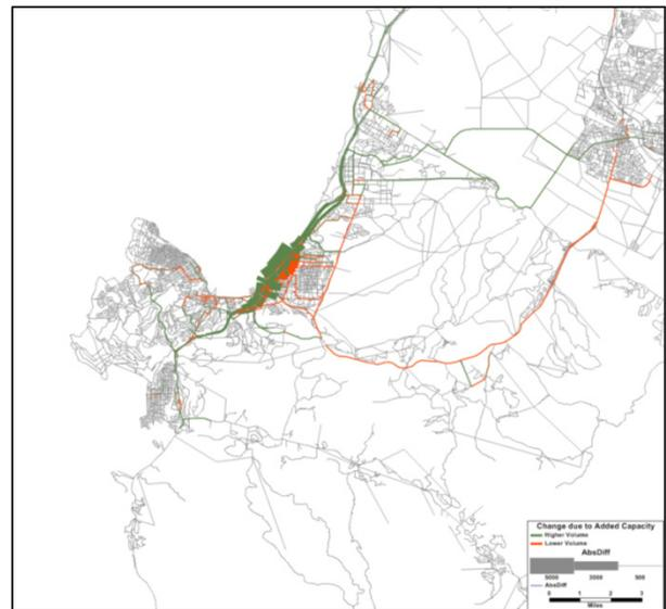
The magnitude, direction and area of influence for the widening is appropriately sensitive for traffic assignment. Distribution and mode choice were not investigated since the widening was limited and few alternatives are available in the corridor.
