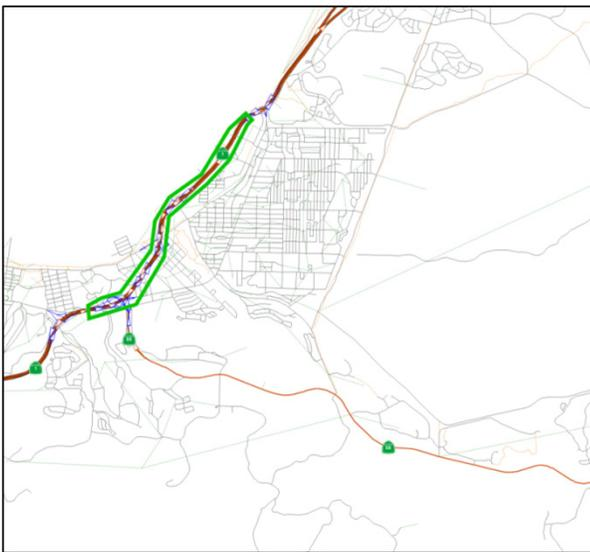
CA 1 was widened within the area highlighted in green. The associated capacity per lane, speed, etc. were automatically updated based on the lookup table by facility type and number of lanes.
